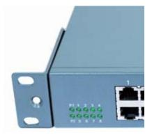
2. Install the long bracket to the other side of the device.
